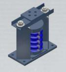
**SLR** restrained spring mounts give the same efficient control of structurally transmitted noise and vibration as do our SLFH and C mounts, but with limited movement. It limit upward travel when weight is temporarily removed and provide safety stops for windy rooftop applications.
